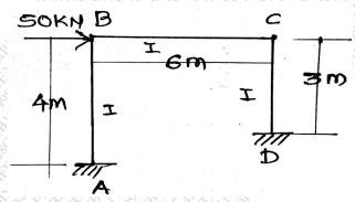
Q.3 Analyse the beam shown in fig. below by using slope deflection method draw BMD & SFD. 15
