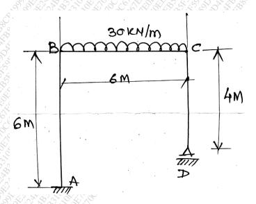
Q.8 Analyse the continuous beam as shown in fig by using KANI'S METHOD. If support B & C 15 sinks by 2mm and 5mm. Take  $E = 200KN/M^2$ ,  $I = 2.5 \times 10^{-5}M^4$
