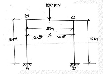
Q.7 Find the end moments of the members of the portal frame as shown in fig by using MOMENT 15 DISTRIBUTION METHOD. Draw BMD.
